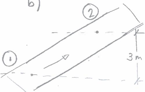
$$\frac{p_1}{\gamma} = 36 \text{ m}, \text{ tubo inclinado e } \Delta N = 3 \text{ m}$$
